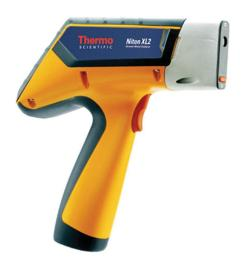
Niton XL2 100G: With point-and-shoot simplicity, you can view the alloy grade and chemistry on the built-in, color, touch-screen display.
